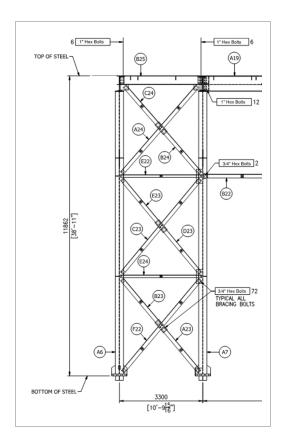
The plan for our crew tomorrow will be to shake out and transport the steel members by truck to the work area. We will also plan to erect and bolt up members C23, D23, E23, and E24. We will use a JLG to help with erection.
