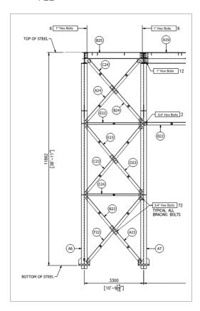
The plan will be to shakeout and transport the steel members by 1/2 ton pickup truck to the work area. You also plan to erect and bolt up members C23, D23, E23, and E24. You will use a JLG to help with erection.
